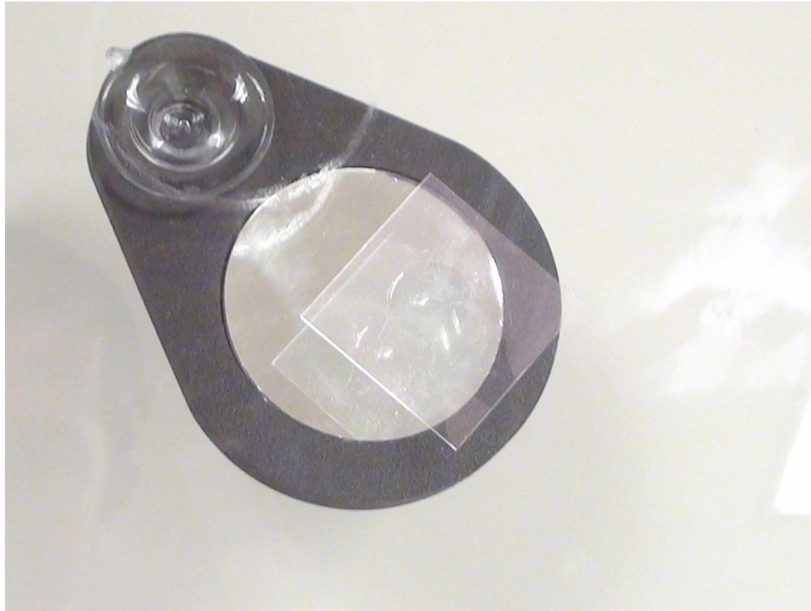
Properly laid curing tab.
